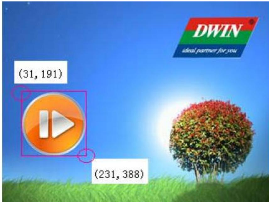
As shown in above picture, the coordinate of the valid button shall be  $31 < x < 231$   $191 < y < 388$ . In general, touch position is obtained by serial port break.
