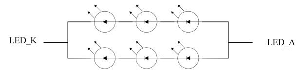
■ The constant current source is needed for white LED back-light driving.
