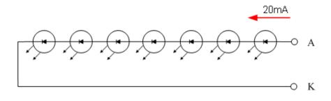
■ The constant current source is needed for white LED back-light driving.
