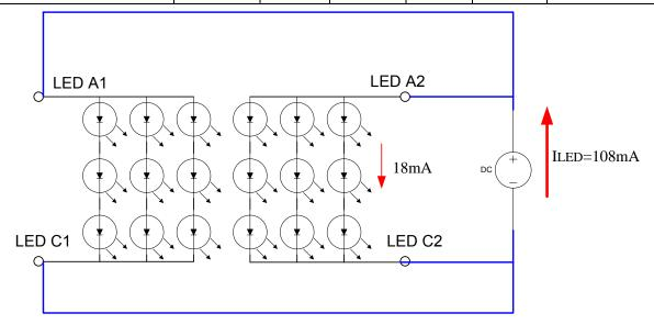
■ The constant current source is needed for white LED back-light driving.
