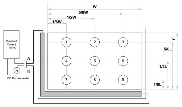
Note3: The Uniformity definition (Min Brightness / Max Brightness) x 100%
