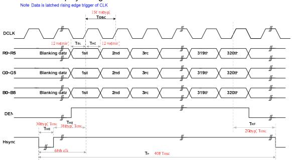
If DEN is fixed to low the SYNC mode is used. Otherwise DE mode is used. When SYNC mode is used if st data start from 68th CLK after Hsync falling.
