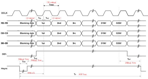
If DEN is fixed to low the SYNC mode is usec. Otherwise DE mode is usec. When SYNC mode is usec. 'st data start from 68th CLK after Hsync falling
