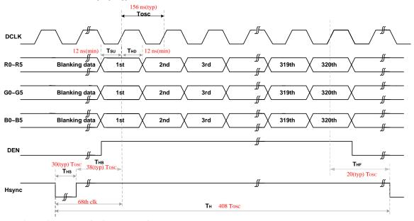
If DEN is fixed to low, the SYNC mode is used. Otherwise DE mode is used. When SYNC mode is used, 1st data start from 68th CLK after Hsync falling
