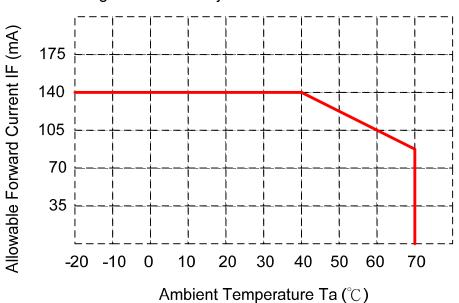
back-light should be adjusted to 105mA max
