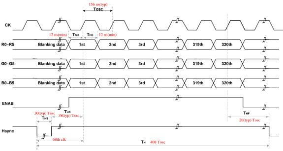
If ENAB is fixed to low, the SYNC mode is used. Otherwise DE mode is used. When SYNC mode is used, 1st data start from 68th CK after Hsync falling
