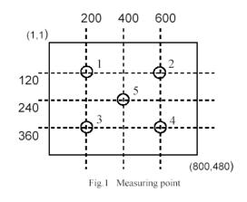
(4) Definition of Luminance Uniformity: Measured Maximum luminance [L(MAX)] and Minimum luminance[L(MIN)] on the 5 points.
