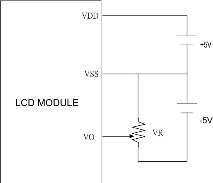
VDD-VO: LCD Driving Voltage
